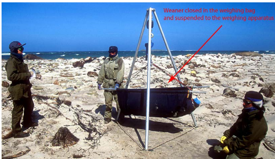
Figure 17 – Weighing of a weaned pup. The canvas bag is connected to the tripod and lifted using a hoist. We usually wait 10 to 30 seconds to let the dynamometer reading stabilize.
