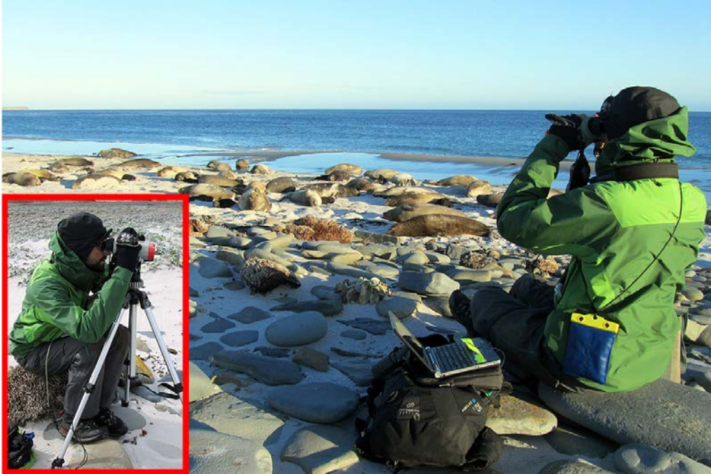
Figure 14 – Use of laser telemetry to map the seals of a harem. The insert shows the Laser Locator mounted on a tripod.
