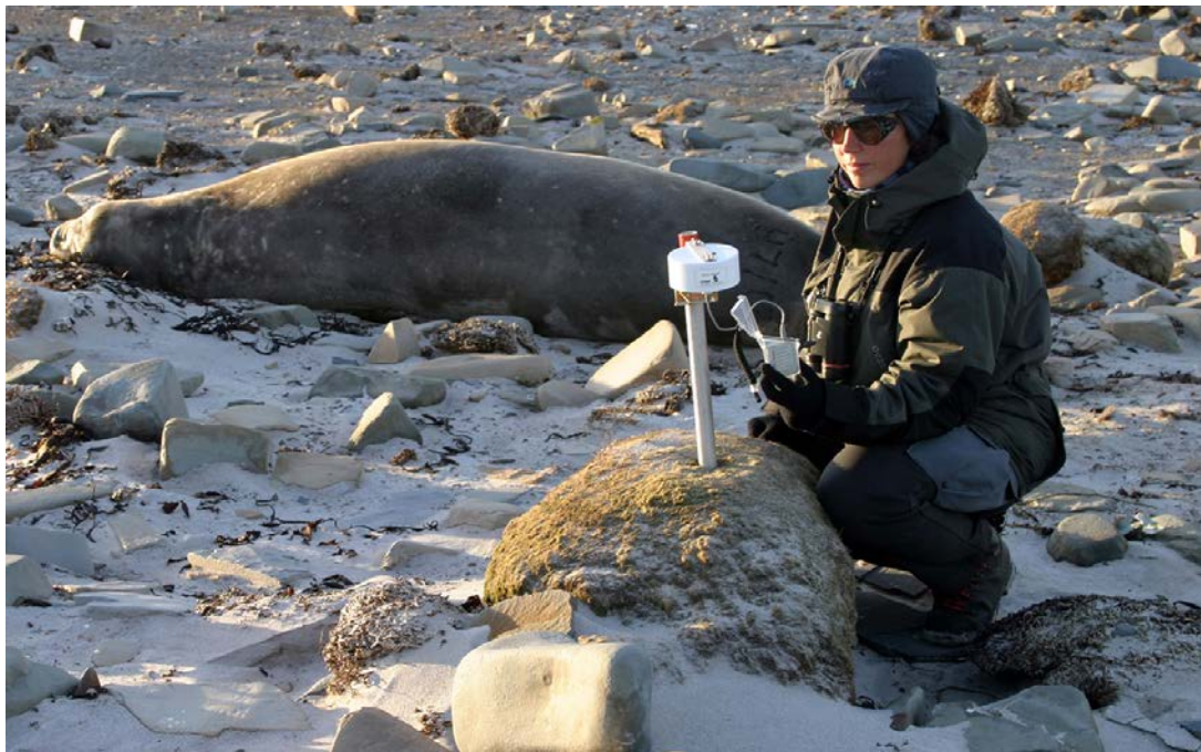
Figure 27 – A datalogger with the rain/sun cover. The logger data (air temperature and humidity) is being downloaded using a dedicated shuttle. Please note the nearby resting elephant seal female.
